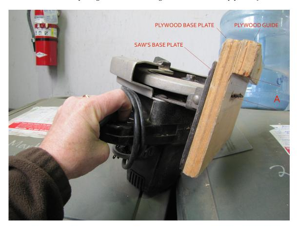
The most crucial measurement is the distance between the bottom of the guide and the center of the saw blade (A in above image).
